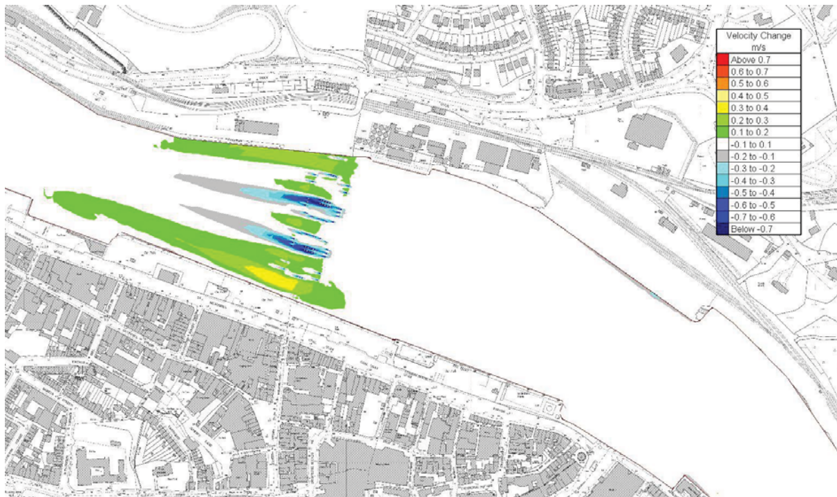
Figure 29 Computed change in velocity magnitude as a result of the bridge – Spring Tide Mid-Flood
