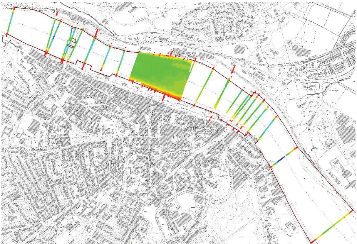
Figure 6 Bathymetric Survey data coverage for Study Reach in vicinity of proposed Bridge crossing
