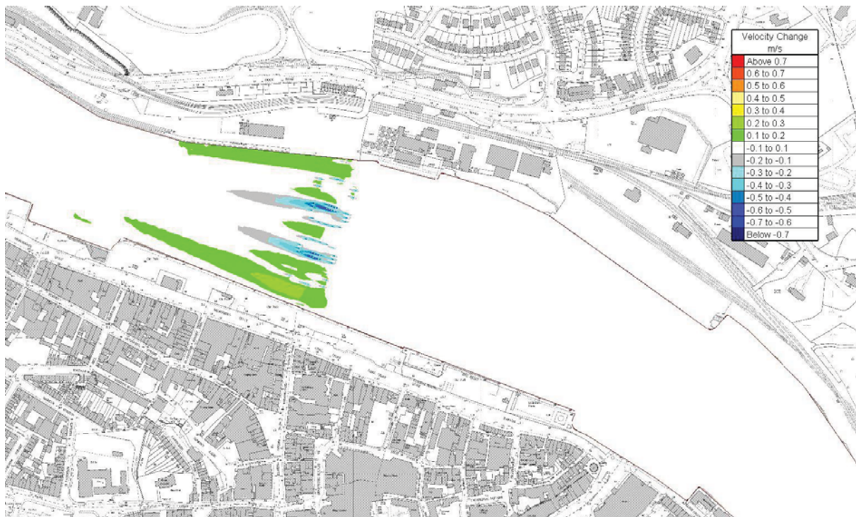
Figure 27 Computed change in velocity magnitude as a result of the proposed bridge – Neap Tide Mid-Flood
