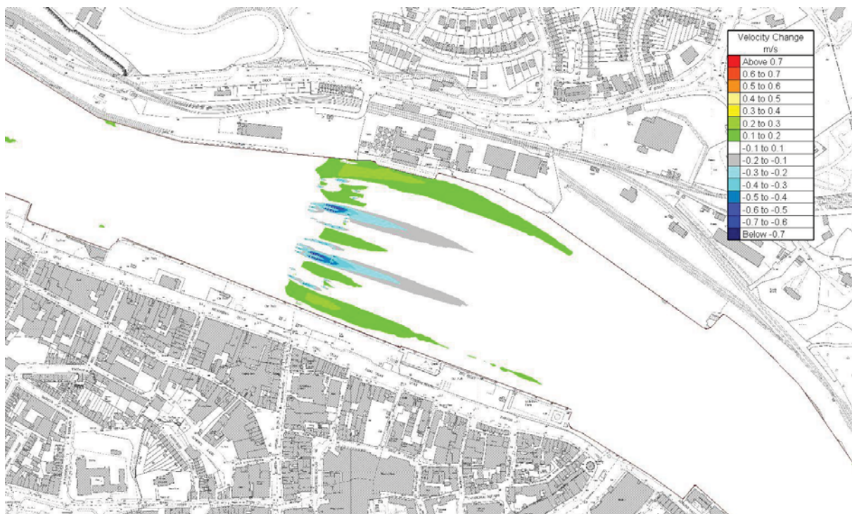
Figure 28 Computed change in velocity magnitude as a result of the bridge – Neap Tide Mid-Ebb
